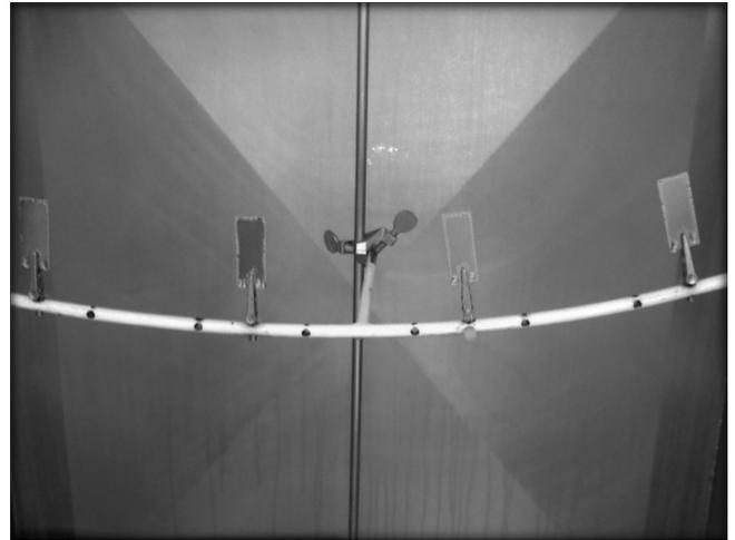
FIG 3 Arched attachment point for virus-inoculated stainless steel target coupons, secured in place by alligator clips inside the spray chamber.
