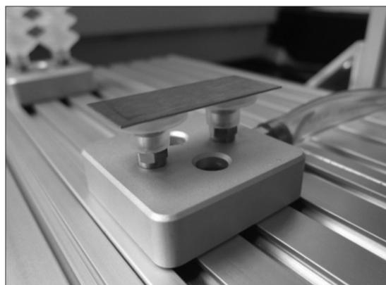
FIG 6 Close-up view of a stainless steel target coupon held in position by vacuum on the stationary platform of a vacuum on the stationary platform of a SAM.
